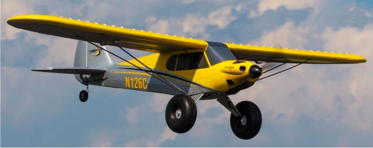
Crafters (which is modern iteration of the classic Piper Super Cub). The HobbyZone “bind and fly” rendition is an EPO foam model weighing in at 2.3 pounds with a 51” wingspan, 480 size motor, 18 Amp ESC, installed micro servos, Spektrum SPM4647 Receiver, Spektrum SPMA3232 Flight Controller and Spektrum SPMA3173 GPS module. The large “tundra” tires make it easy to lift off and land in a grass field and it will run for 6 minutes on a 3S-2200 LiPo battery.
